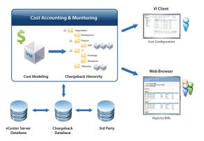
VMware vCenter Chargeback is based on a flexible hierarchy and cost models that can be customized to the organization's requirements.
